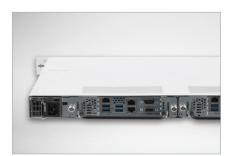
**1200W Removable PSU** Ample wattage in a low-profile power supply that easily supports both processor boards.
