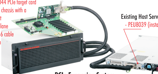
PCIe Expansion System (Integrated Target Chassis & Existing Host Server)
