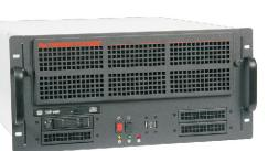
Trenton TVC5401 Video Controller Shown with 18-slot backplane and a single processor SBC
