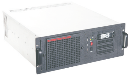
Trenton TRC4008 Rackmount System Shown with a 14-slot backplane and one SBC
