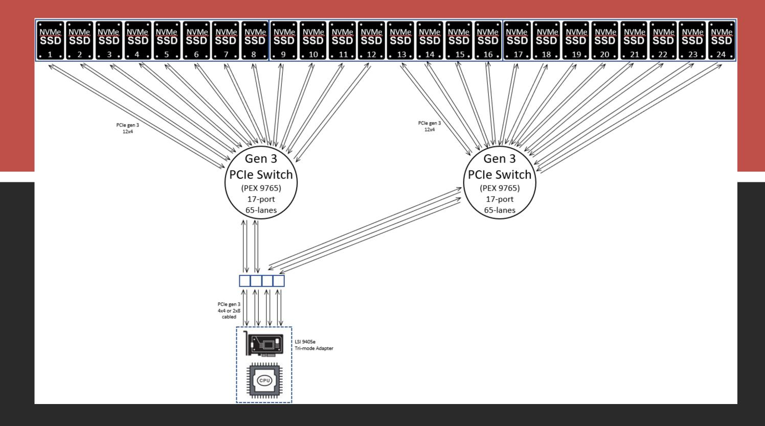
There are several other use cases for the Trenton Systems JBOF System. Here you can see an example where the host computer only has one PCle expansion card. While not as ideal for bandwidth or redundancy, this lowers the total cost of the system.
