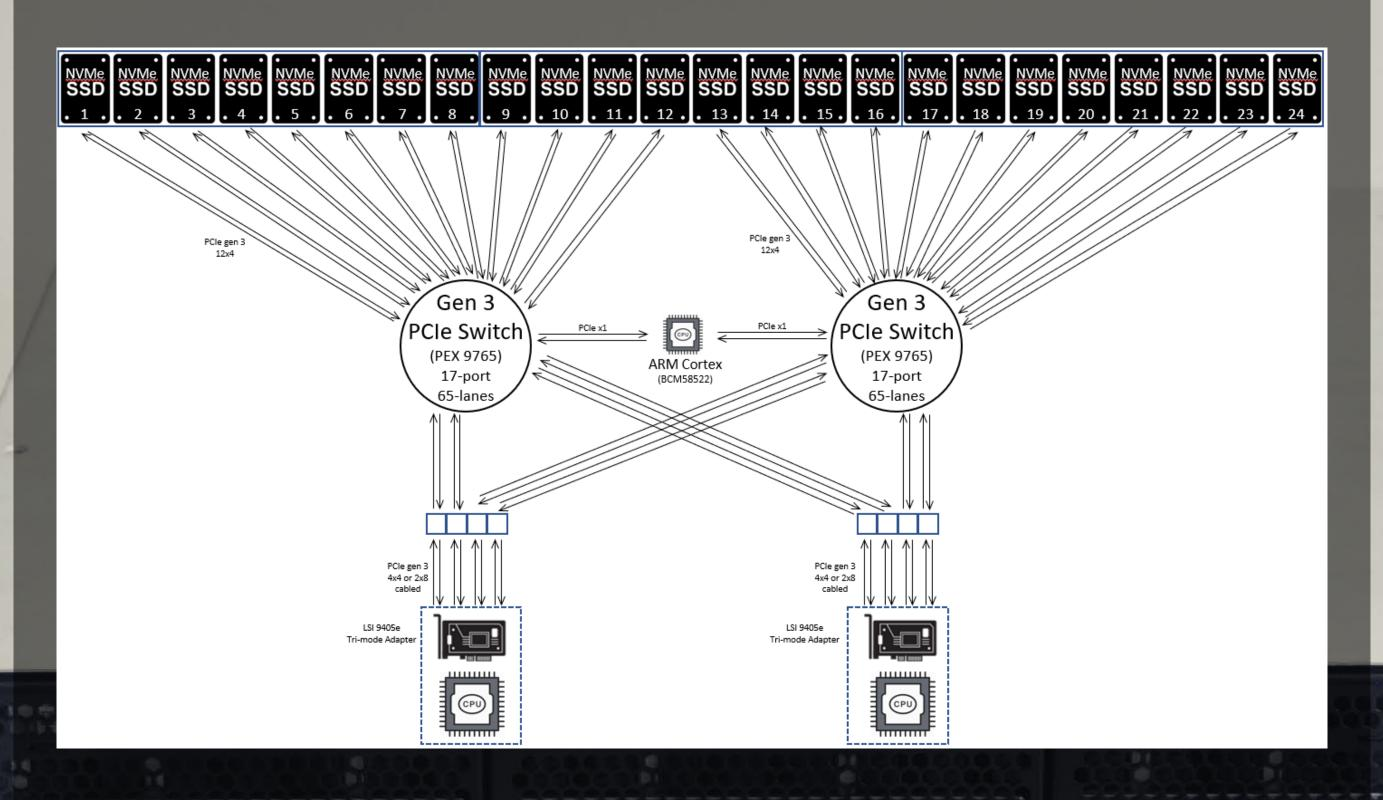
While the max theoretical throughput is 27GB/s (8 drives running at 3.375GB/s each), actual results depend on many different realworld factors (i.e. packet size, load balancing between multiple CPUs, drive performance, etc). For many of Trenton Systems tests, we have used the Intel DC P4510 U.2 NVMe drives. These Intel drives are ideal for applications where high-performance and reliability is required, but other U.2 NMVe drives would also perform well in this Trenton Systems JBOF system.
