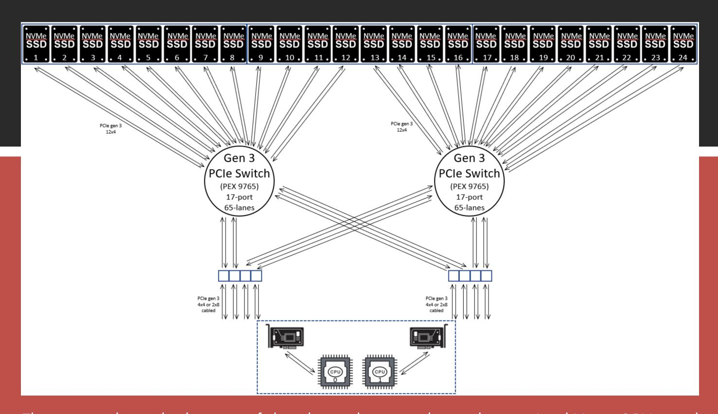
The rectangle at the bottom of the above diagram shows the two Intel Xeon CPUs each connected to a PCIe host expansion board. The host cards could be plugged into almost any rackmount or desktop class computer which makes this JBOF truly agnostic to the host computer. Note that some consumer-class computers may have BIOS limitations (i.e. memory space) so it is important that you consider the proper host processor board.
