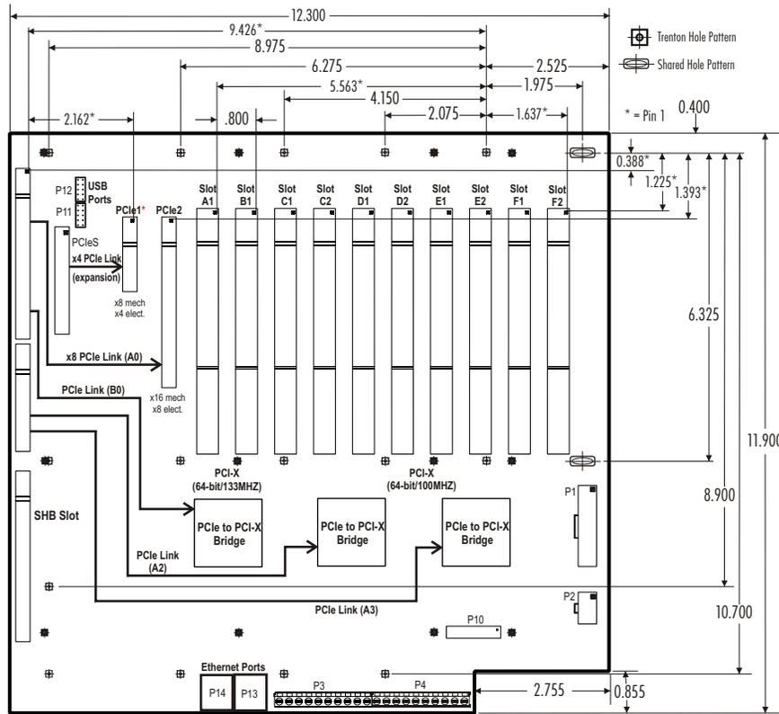
\*PCIe1 slot functionality requires an IOB31 installed on the SHB
